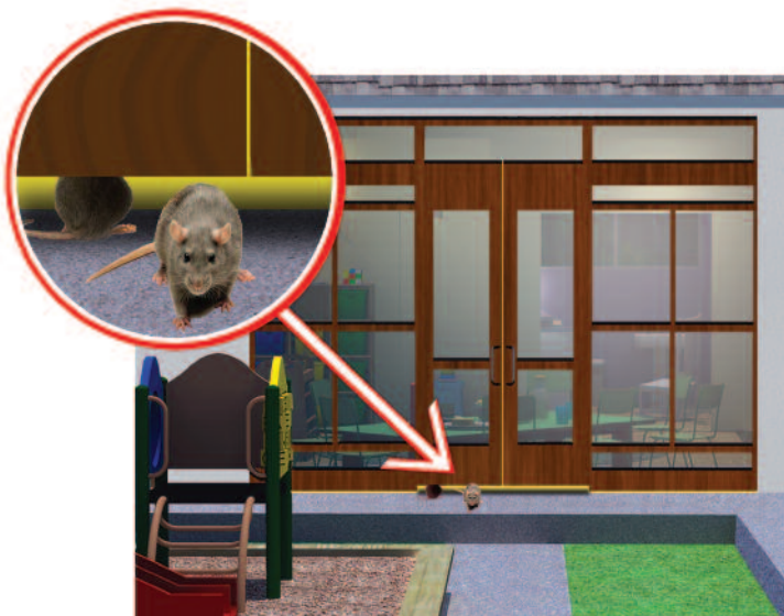
Install door sweeps.
